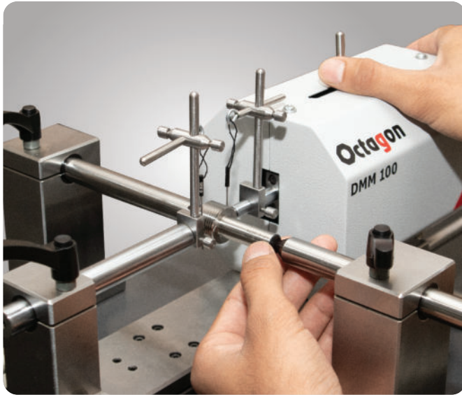
Cy. Thread Plug Gauge measurement (2 wire method)
