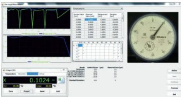
Windows based program for evaluation of measuring errors, a laptop or PC. Online Data acquisition, Data recording, certificate generation.
