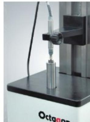
Calibration of Electronic Inductive Probe
