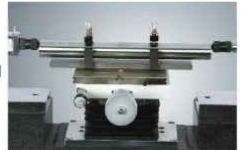
Length bar measurement : Hold on table by using holding attachment
