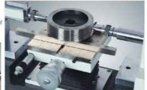
Cy. Thread Plug Gauge Measurement of Effective diameter Below 40 mm : Hold in Vee block holder
