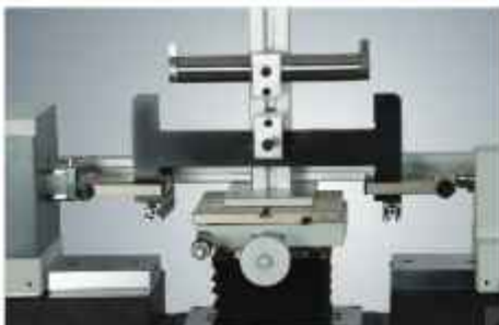
Snap Gauge ( I type) measurement : Hold on universal holder
