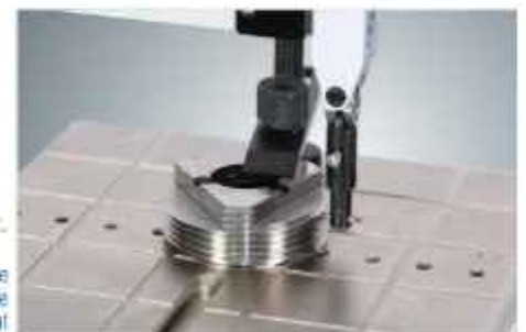
Measurement of effective diameter by T Shape Ruby Stylus Two axis bi-directional probing
