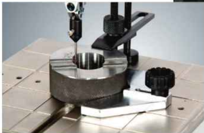
Taper ring gauge measurement : Using a Single Ruby Ball Stylus with bi-directional probing system of single arm measuring attachment
