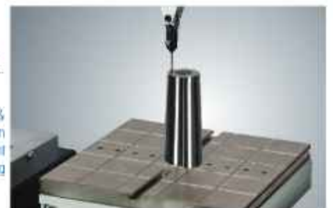
Taper Plug gauge measurement : Using a Single Ruby Ball Stylus with bi-directional probing system of single arm measuring attachment
