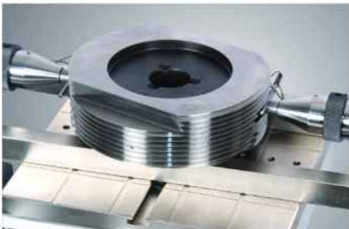
Measurement of effective diameter by thread measuring wires
