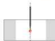
Measurement of internal diameter by using single arm measuring attachment with one axis bi-directional probing
