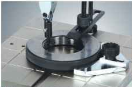
Cy. Measurement of effective diameter by using single arm measuring attachment & Precision Ruby T-Shape styl
