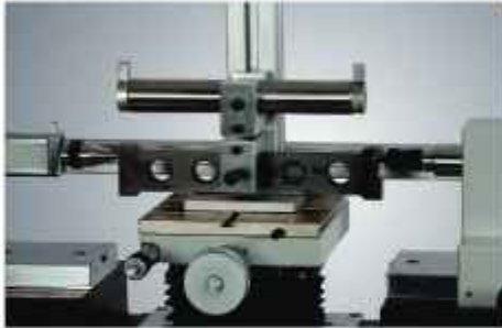
Plug Gauge (plate type) measurement : Hold on universal holder
