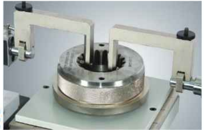
Spline ring gauge measurement by using fixed dual arm and precision spherical styli : Hold on floating table.
