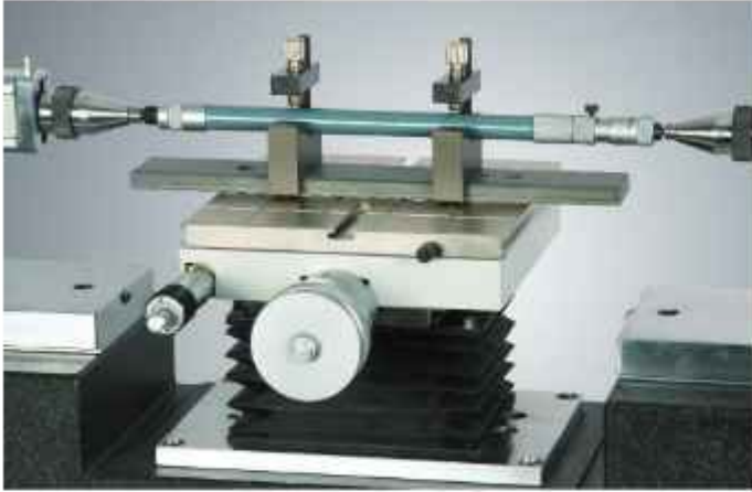
Internal Micrometer (2 point) Calibration : Hold on table by using holding attachment
