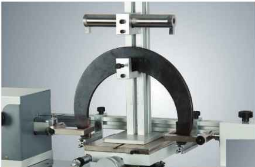
Snap Gauge C Type (above 300 mm) measurement : Hold on universal holder
