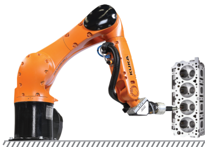
Non contact Pneumatic Probe with multiple jets
